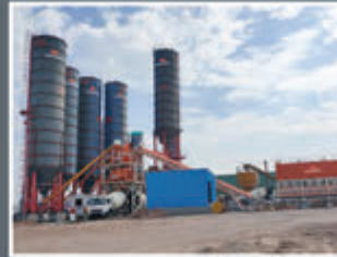
MCP BIN-90 Concrete Batching / Mixing Plant
