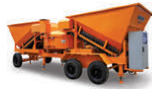
Mobile Concrete Batching / Mixing Plant
