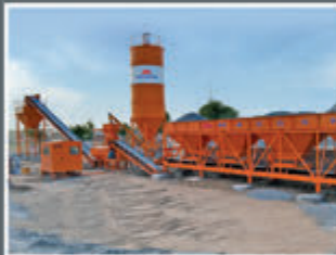
Wet Mix Macadam Plant with CTAB System
